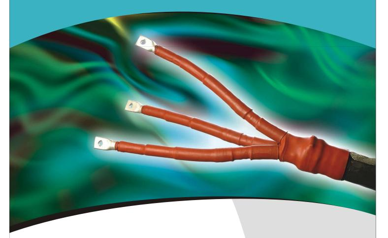
M-Seal heat shrink (HS) Terminations up to 36kV, are specially designed for conditions where the terminations are exposed to precipitation, outdoor sunlight, extreme climatic variances and heavily polluted areas. The specially engineered kits also take care of the typical partial discharge and surface corona phenomenon for all power cables under challenging service conditions.
